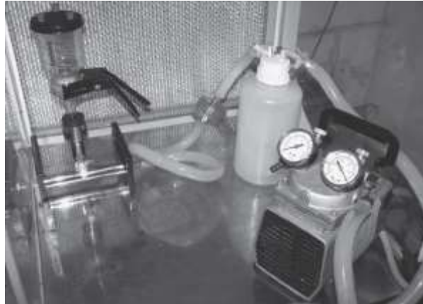
Fig. Experimental set-up for low-cost pressure filtration of coconut water ( Indian Patent filed for ).
